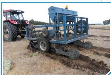
CommVeg seeder enables optimal seed placement, which is critical on light sandy soils that are unable to retain moisture around the seed. For more information contact NSPNR.
