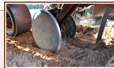
Soil preparation achieved with the CommVeg seeder. The machine was travelling from left to right and the image shows the view behind the scalper, showing clean dirt being ripped (spring tyne), small tillage disks and the first wheel of the floating seeder arm which places the seed and presses the seed sowing trench.
