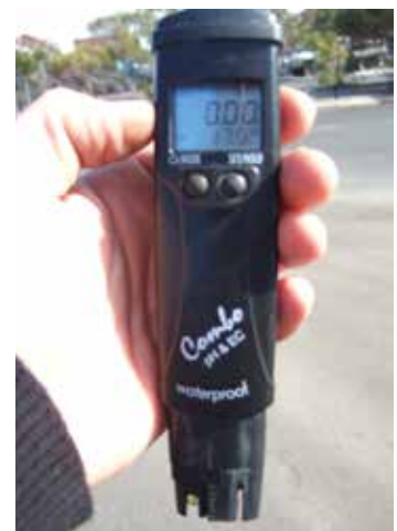
A waterproof handheld 'EC Salinity and pH' meter. Note: it is important to calibrate and check the instrument for accuracy regularly.
