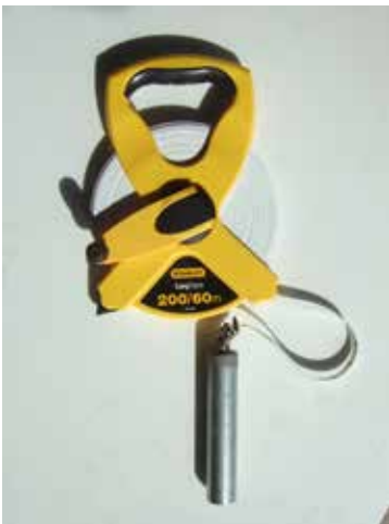
PVC or metal 'plopper' attached to a graduated measure tape measure for testwell/piezometer depth measurement
