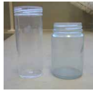
Two straight sided plastic jars with graduated measures (1 x water sample jar and 1 x EC 1:5 soil testing jar).
