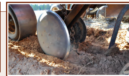
Soil preparation achieved with the CommVeg seeder. The machine was travelling from left to right and the image shows the view behind the scalper, showing clean dirt being ripped (spring tyne), small tillage disks and the first wheel of the floating seeder arm which places the seed and presses the seed sowing trench.
