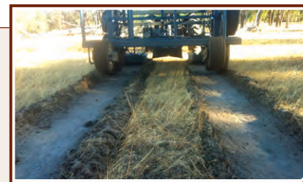
An ideal scalp created by the CommVeg seeder. 5-7cm of soil being removed from the centre of each scalp, grading to 0cm on the outer sides of each scalp line.
